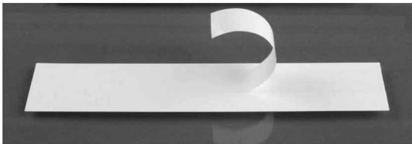
Fig. 3.1 A typical backing with part of release liner partially peeled back. (Photo courtesy of G&L Precision Die Cutting, Inc. San Jose, CA, USA)
