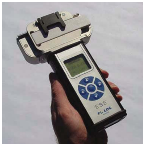
Fig. 9.7a Battery-operated handheld lateral flow reader prototypes by ESE for colorimetric readout using colloidal gold beads or color latex beads ( GoldScan ) and fluorescence labels ( FluoScan )
