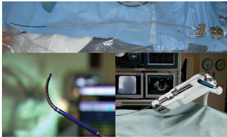
Figure 6 Steerable guide catheter inside a steerable sheath that A consists of an 8.5F through lumen. It mounts on portable robotic catheter manipulator ( B ) and has 6° of freedom ( C )
