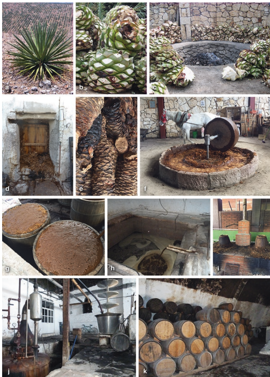
Fig. 16.4 Mezcal elaboration process. (a) Agave angustifolia . (b) Raw agave heads or piñas . (c) Pit oven filed with stones. (d) Brick oven. (e) Cooked agave heads or piñas . (f) Rudimentary mill or tahona . (g) Fermentation of cooked agave must with fiber in wooden vats. (h) Fermentation of agave must without fiber in a brick tank. (i) Distillation of fermented agave must in a rudimentary still. (j) Arab type still. (k) Mezcal aging in oak barrels (optional)
