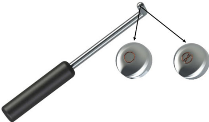
Fig. 8.2 A pencil probe. Enlargements of the tip area show either an absolute coil configuration (left) or a differential coil configuration (right)
