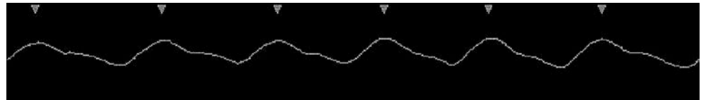
Fig. 2.3 Signal from a peripheral pulse monitor, with demonstration of triggering with each pulse cycle
