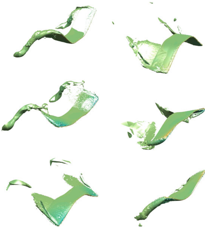
Fig. 13 Visualization of the flow field around wing with flapping motion corresponding to the solution of the optimization problem in (50). The color shows the pressure field on the wing surface as well as on an isosurface of the streamwise vorticity. Snapshots (top to bottom, left to right) taken at equally spaced time increments during the second period that correspond to times t = 5.0, 5.83, 6.67, 7.5, 8.33, 9.17
