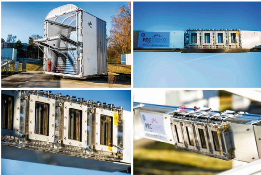
Hydrogen Production from Photoelectrochemical Water Splitting, Fig. 23 Image of the demonstrative PEC/PV prototype module hosting four new “PortoCell,” which contains photoelectrodes and silicon PV cells with an active surface area of 50 cm 2 each. The prototype has
