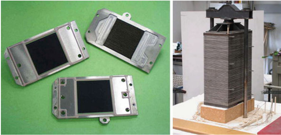
Solid Oxide Fuel Cells: Sustainability Aspects, Fig. 20 Single repeating units and 15 kW class stack of the stationary SOFC design
