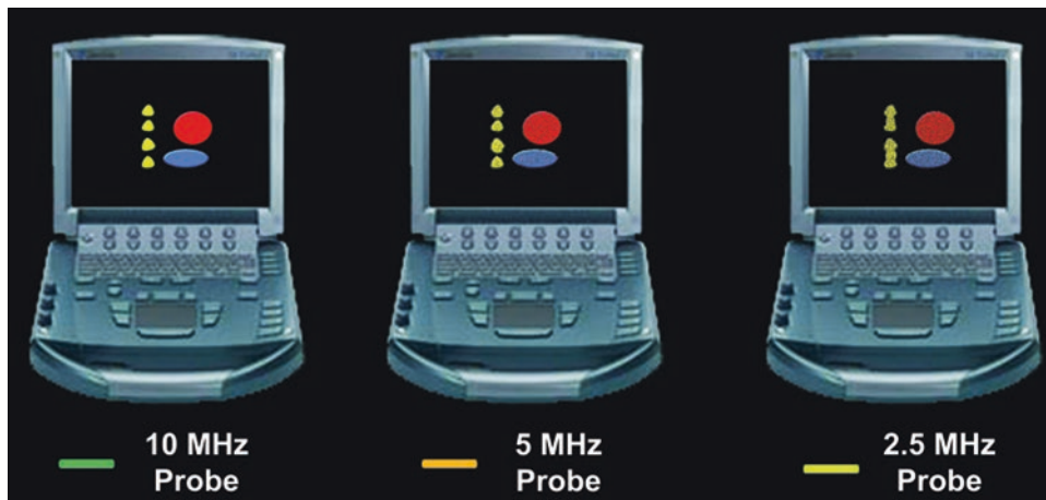
Fig. 3.2 Axial resolution denotes the ability of the ultrasound machine to visually separate two structures lying atop one another (y-axis) in a direction parallel to the beam. As frequency increases, axial resolution increases, but depth of penetration decreases. Low-frequency waves
