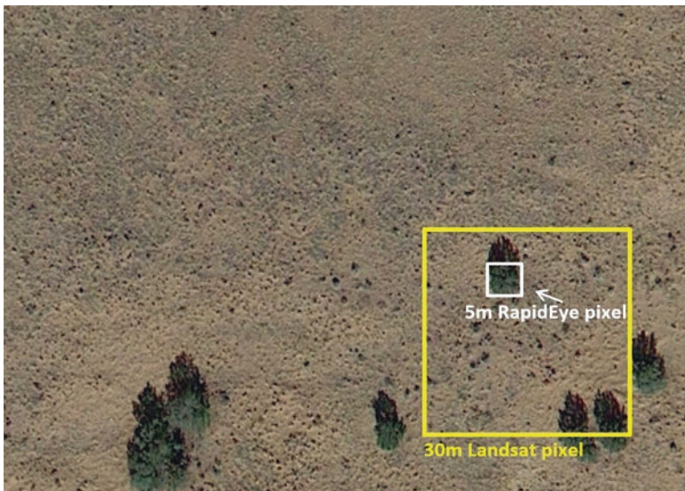
Fig. 6 Comparison of spatial resolution of satellite image sources, Landsat TM (30 m) versus RapidEye (5 m), from a grassland system with juniper encroachment east of Grants, New Mexico, USA (Earth 2014a)
