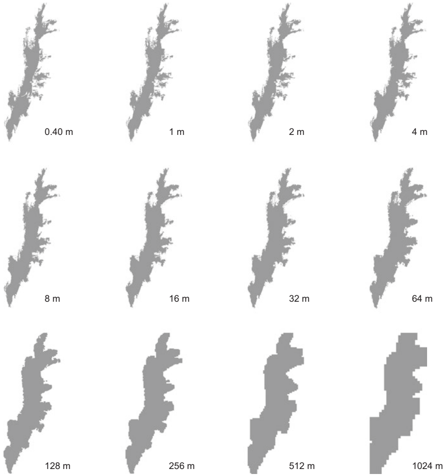
Fig. 6 The same fire footprint depicted at spatial resolutions ranging from 0.4 to 1024 m. In each case, estimates of the area, perimeter, number of spot fires, and the area of the spot fires are affected. Figure 7 depicts these changes graphically
