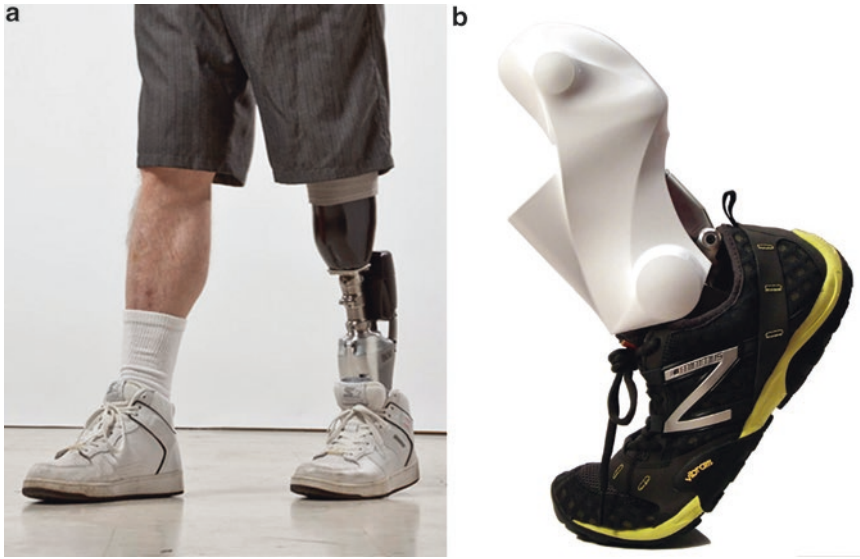
Fig. 4.14 Actively powered foot-ankle systems: (a) the BiOM® Ankle System (Image courtesy of BiOM) and (b) the Odyssey ankle (Image courtesy of SpringActive, Inc.)
