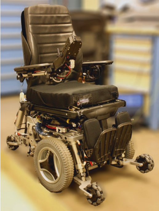
Fig. 2.3 The Mobility Enhanced Robotic Wheelchair (MEBot) is an advanced wheeled mobility platform designed to provide exceptional indoor and outdoor mobility for people with impaired lower and upper extremity function. The MEBot provides such seating and accessibility features as fore/aft tilt, lateral tilt, recline, and elevation within a small footprint for indoor mobility and activities of daily living. In addition, it provides remarkable outdoor mobility to include curb climbing, self-leveling over uneven terrain, and crawling (Courtesy of Human Engineering Research Laboratories (HERL), http://www.herl.pitt.edu/ )
