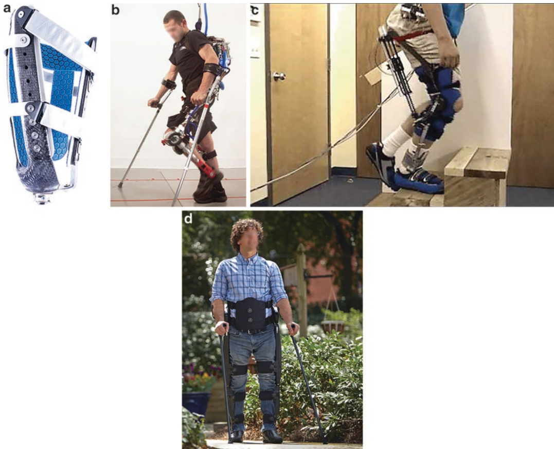
Fig. 5.1 (a) Socketless socket for a transfemoral prosthetic (Courtesy of Martin Bionics) (b) MinaV0 exoskeleton (Courtesy of Florida Institute for Human Machine
