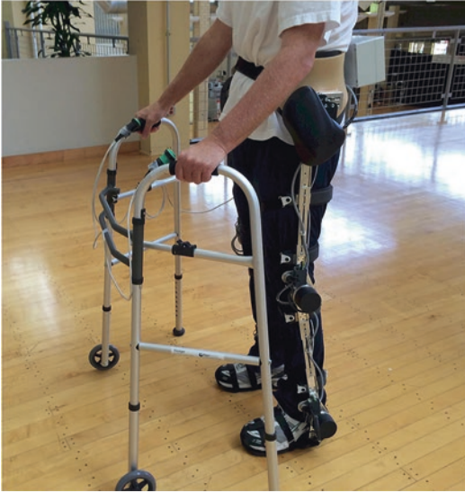
Fig. 5.13 Stroke patient using H2 exoskeleton at the beginning of one training session (Courtesy of Journal of Neuroengineering and Rehabilitation)
