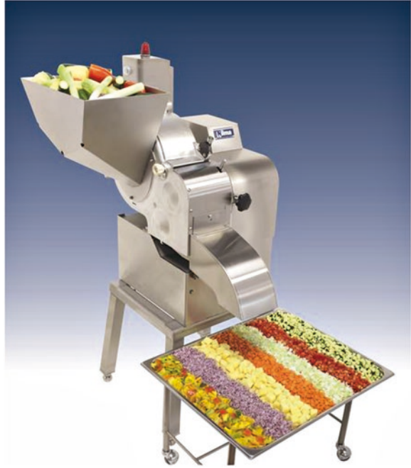
Fig. 3.15 A various size and shape cutting machine for fruits and vegetable
