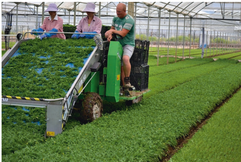
Fig. 11.6 Mechanical harvest of “baby leaf” wild rocket ( Diplotaxis tenuifolia L.) grown under protected environment
