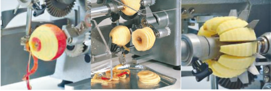
Fig. 3.12 Automatic apple washing, peeling, coring, and slicing machine
