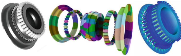
Fig. 11.7 Frictionless roller bearing of wind generator
