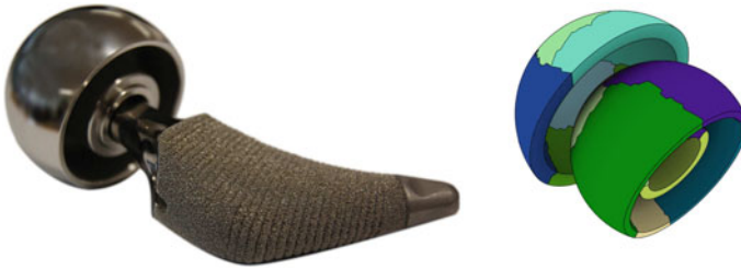
Fig. 1.8 Hip joint substitute ( left ) and its model decomposed into subdomains ( right )
