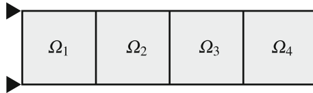
Fig. 19.2 2D cantilever beam decomposed into four subdomains
