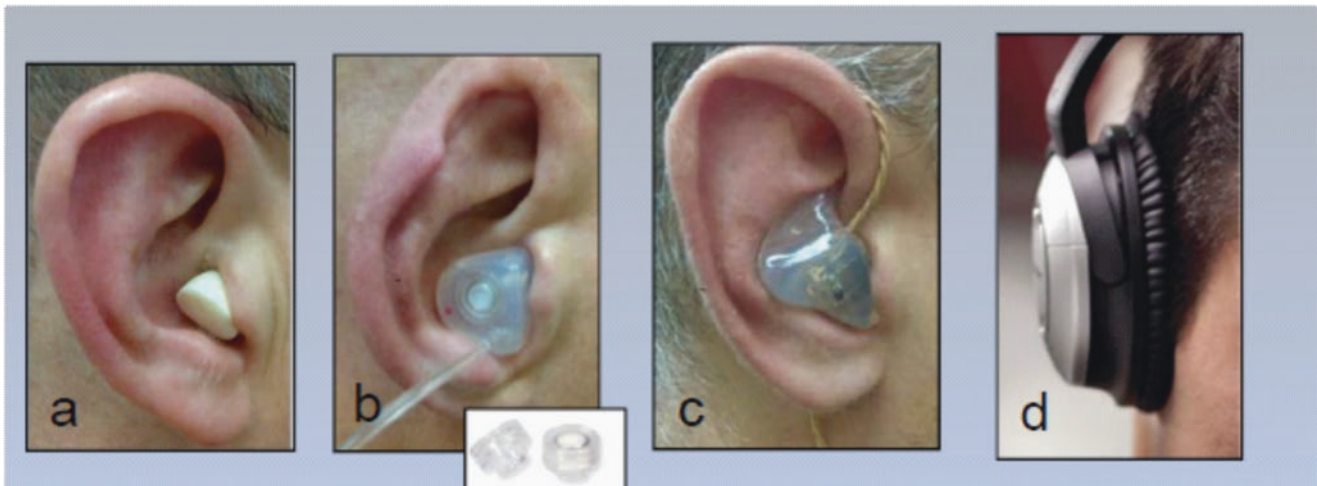
Fig. 6.20 Examples of hearing protective devices used on the ISS. (a) Disposable foam earplugs, which attenuate more high frequency sounds than low frequency sounds. (b) Custom-made silicone earplugs (often referred to as “musician’s earplugs”) and filters that attenuate sounds (by 15 or 25 dB) uniformly across all frequencies. (c) Custom-made silicone ear monitors, which have two high-fidelity speakers, used to attenuate ambient sounds while producing acoustic stimuli for the On-Orbit
