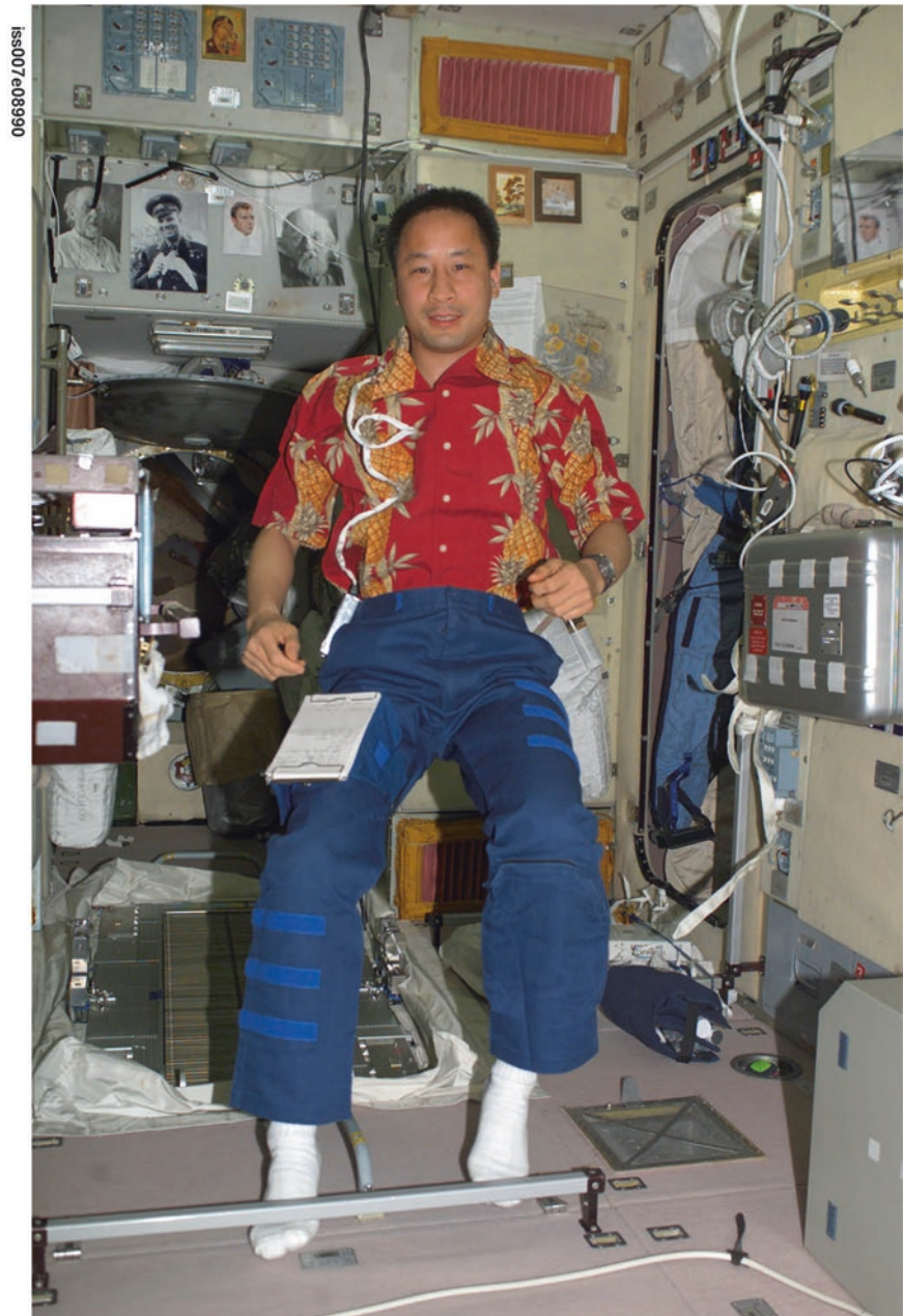
Fig. 6.8 ISS Acoustic Dosimeter, which shows a crew member wearing a dosimeter at the belt with the microphone clipped to his collar (Courtesy of NASA)
