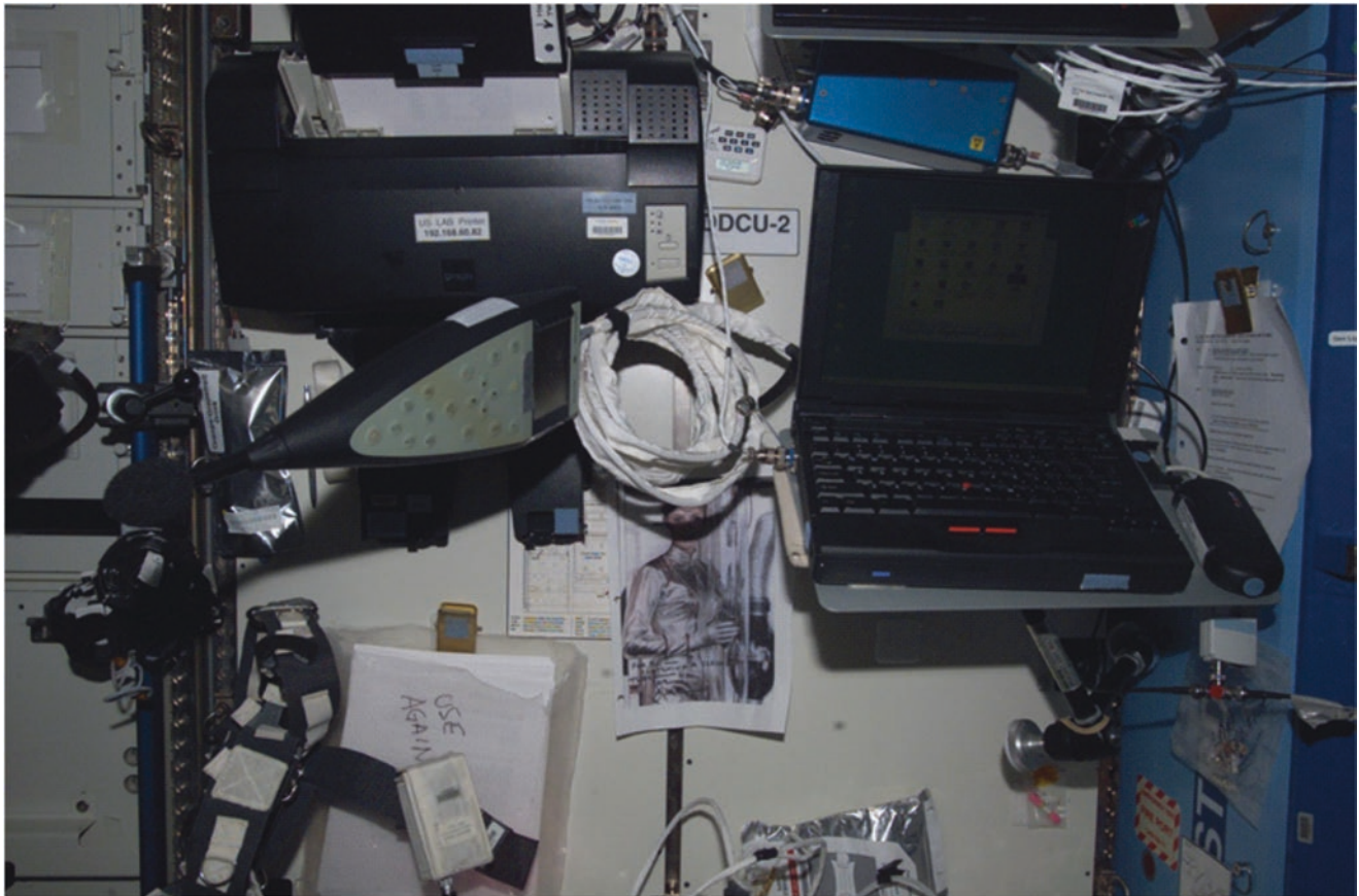
Fig.6.7 ISS Sound Level Meter (SLM), connected to Space Station Computer (SSC) for download (Courtesy of NASA)
