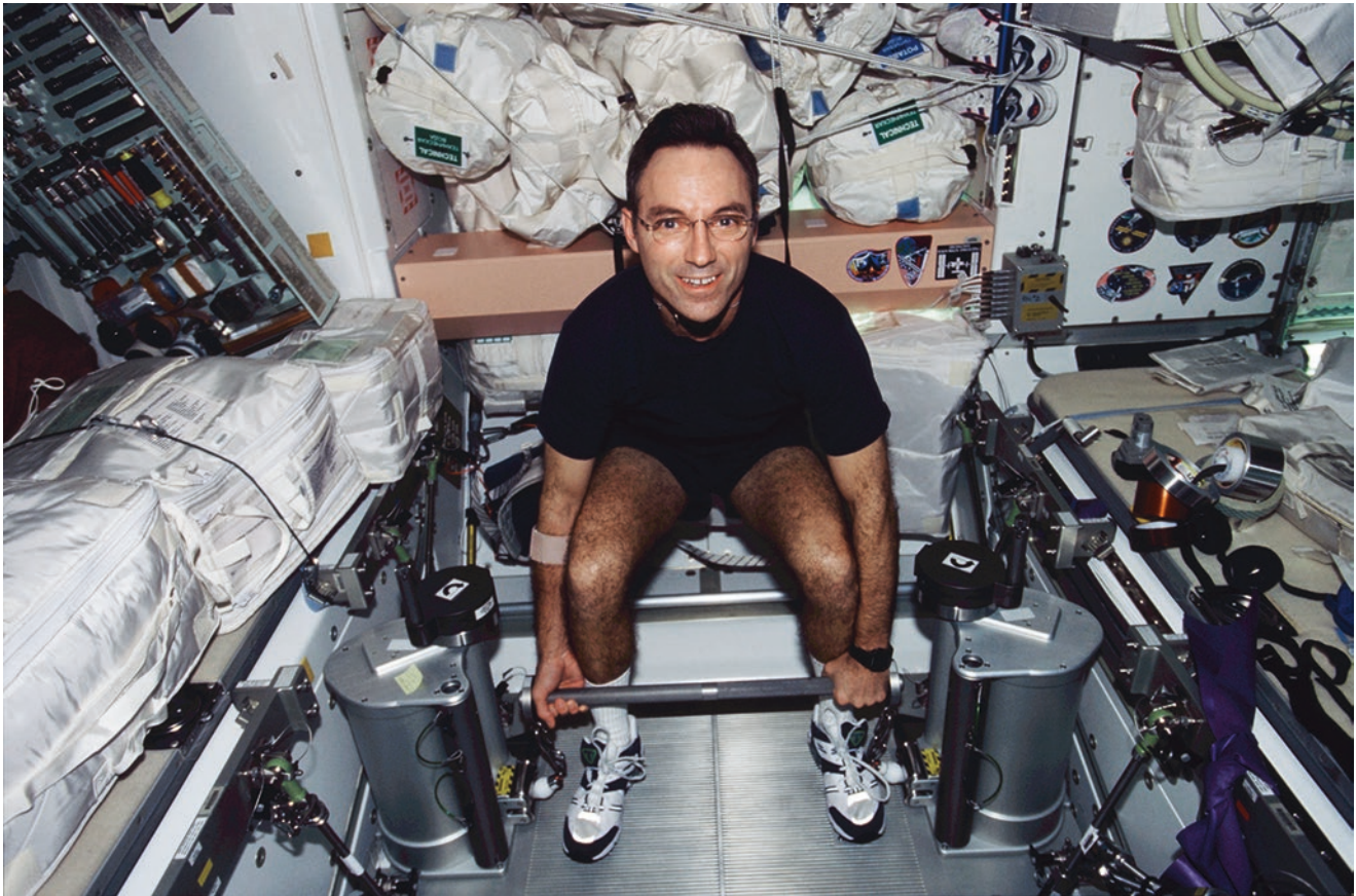
Fig. 13.6 Astronaut Carl Walz uses the short bar on the interim Resistive Exercise Device (iRED) (courtesy of NASA)
