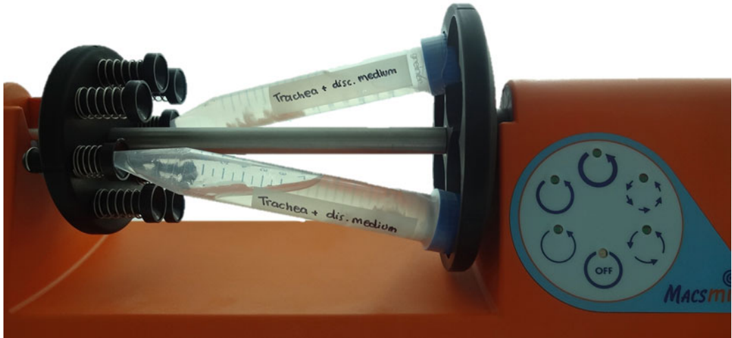
Fig. 3 MACSmix™ tube rotator. The trachea pieces were submerged in dissociation medium and incubated for 24 h at 4 °C
