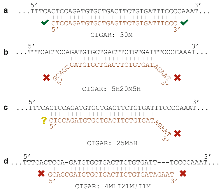
Fig. 6 Example alignments of read sequences ( bottom ) to reference sequence ( top ) illustrating cases when read mapping ends are ( checkmark icon ) and are not ( cross icon ) appropriate to consider by the FragSeq algorithm. To simplify the example, reads are 30 bases long and we assume that 5' and 3' ends are relevant (see Note 14 ), i.e., the reverse transcriptase copied the RNA fragment to cDNA in its entirety and adapter sequence is trimmed, like read1 in Fig. 3; these assumptions are not valid for all cDNA library preparation strategies. CIGAR alignment strings are shown (see Note 21 ). Vertical lines denote a sequence match. (a) A good alignment that includes both read ends. The single sequence mismatch occurs far away from the ends, so the ends are still useful for FragSeq. (b) The alignment algorithm was unable to align read ends, rendering them useless for FragSeq; however, the middle of the read is well-aligned and potentially useful for other bioinformatics analyses. This may occur if adapter sequence has been stripped incompletely, if the read is chimeric, or if the read is mapped to the wrong locus (can occur if part of the locus is a repetitive element). (c) Only the 5' end of the read is reliably aligned. Although the lack of alignment at the 3' end makes the entire mapping suspect, the aligned 5' end may still be useful for FragSeq (see Note 22 ). (d) Neither read end is reliably aligned. Such alignments should be discarded prior to input to readsToStruct.py (see Note 12 )
