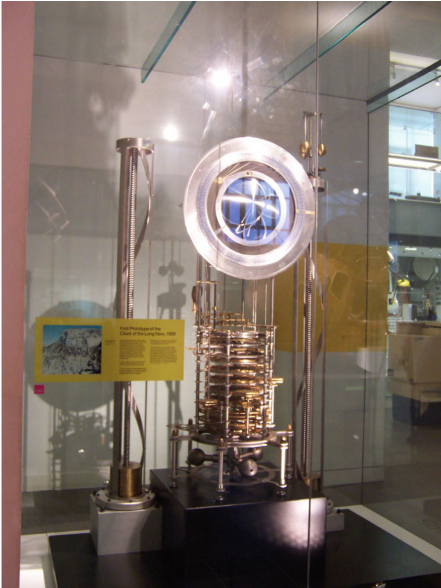
Fig. 3.13 First prototype of the 10,000 Year Clock (1999) on display at the Science Museum in London. The clock ticks once a year. Courtesy of Pkirlin at en.wikipedia.org
