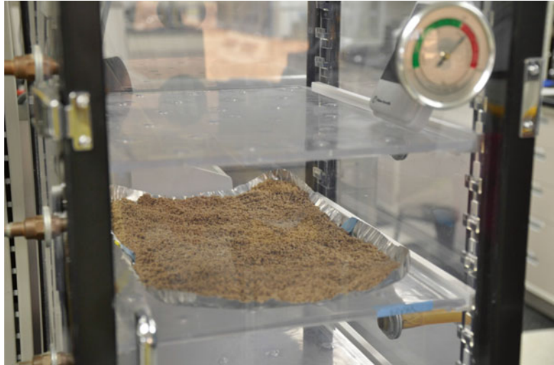
Fig. 5 Microsclerotial granules of Metarhizium brunneum being air-dried in our drying chamber by spreading a thin layer of the DE-microsclerotia mixture on aluminum foil and allowing air to flow over the microsclerotial granules
