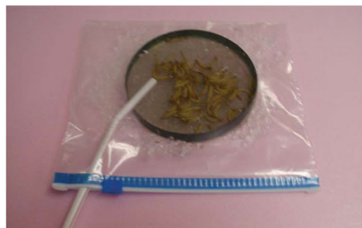
Fig. 7 “Gel System” setup with entomopathogenic nematode infected Tenebrio molitor larvae on a screen on top of a polyacrylamide gel (USDA-ARS)
