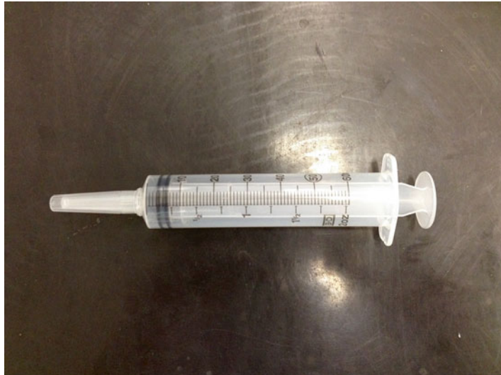
Fig. 4 Photo illustrating the type of syringe used for collection of the fecal material. It is important to use a wide-bore syringe so that the syringe does not “jam.” Although the vast majority of large particulate matter is filtered out with the gauze, some of the fecal sediment that goes through the gauze can still cause the syringe to occlude if a wide-bore syringe is not used
