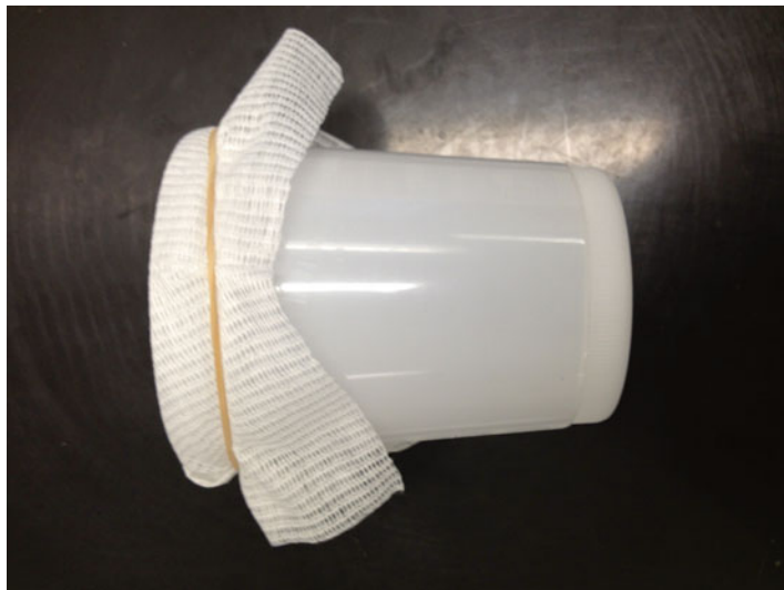
Fig. 3 Photo illustrating how to secure the gauze to the disposable plastic container for filtration of the fecal material
