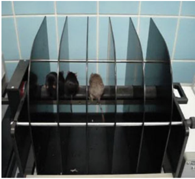
Fig. 2 Photograph of a 5-lane mouse RotaRod. On the right side is a brief overview over the test
