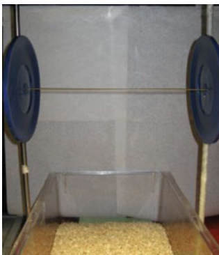
Fig. 4 Photograph of hanging wire setup. The function of the plate-shaped dividers on each side is to prevent the rodent to escape the test setup. On the right side is a brief overview over the test
