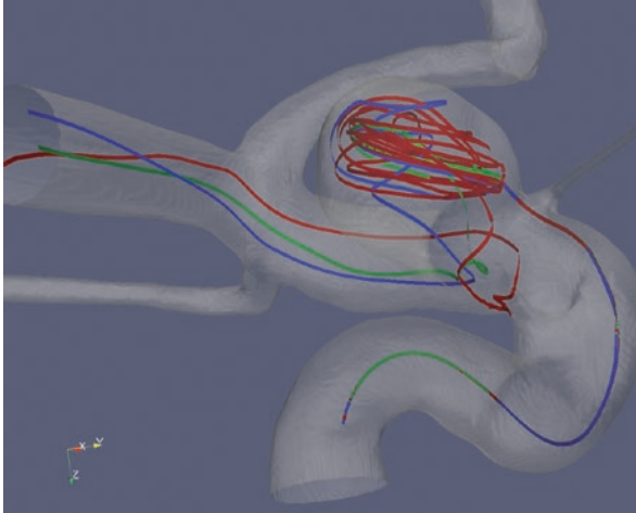
Fig. 17.1 Trajectories of three particles ( red, green, blue ) travelling through the transient flow field of a real aneurysm. Despite the small initial distance between the particles (within 1\ \mu\text{m} ) they travel along substantially different paths. The inlet is towards the bottom of the image, the three outlets are on the top and on the left side of the figure
