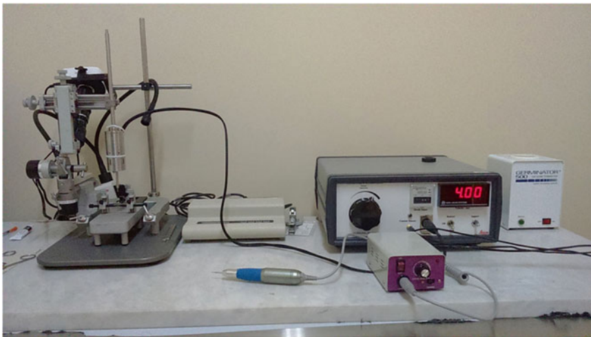
Fig. 3 Controlled cortical impact (CCI) apparatus. A computer-assisted model that induces TBI in the cortex
