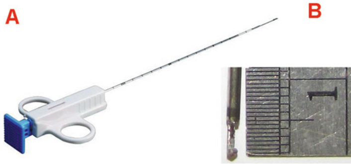
Fig. 2 Biopsy needle to harvest the SVZ from rat brain. (a) A semi-automatic biopsy needle. (b) The tip of the needle that has been re-designed to have a 3 mm cutting window
