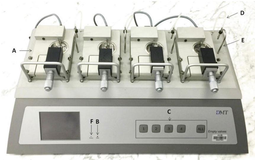
Fig. 4 Multi-wire myograph system (620 M, DMT, Aarhus, Denmark). The system is composed of (a) multi-wire myograph unit, (b) heat indication, (c) valve buttons myo-interface display, (d) gas tube, (e) suction tube
