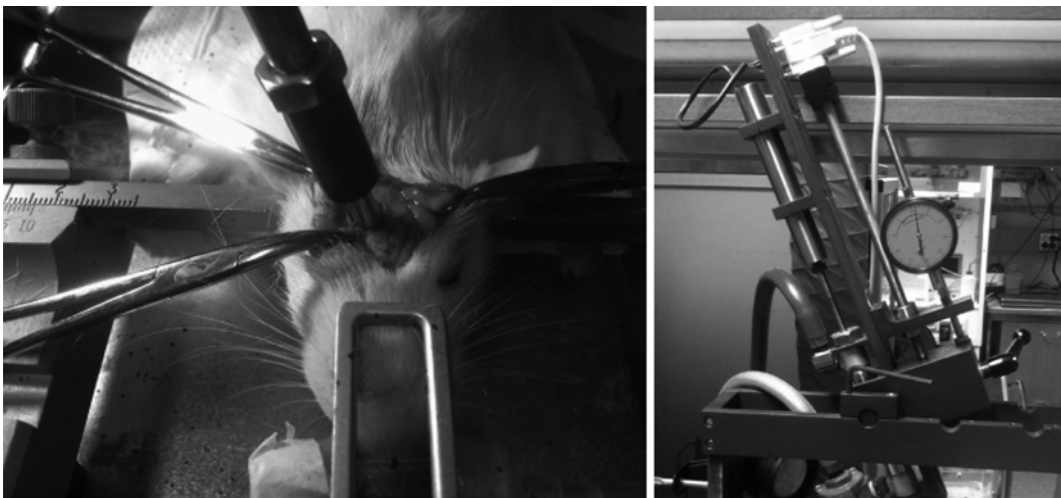
Fig. 3 CCI procedure. Following cleaning of the scalp, a midline incision is made. Following craniotomy made with a dental drill, a 5 \times 6 mm (rats) or 4 \times 4 mm (mice) craniotomy centered over the right parietal cortex is made. The piston ( left ) is gently attached to the exposed dura. To the right , the CCI apparatus including the micrometer gauge is shown
