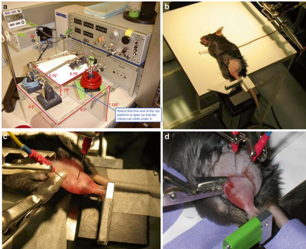
Fig. 4 (a) The custom in vivo platform with dimensions. (b) Optimal placement of the mouse on the platform. The mouse position is secured with adhesive tape, and the self-adhesive temperature probe lies underneath the animal. (c) Appropriate electrode placement on either side of the peroneal nerve for dorsiflexion. (d) Appropriate electrode placement on either side of the sciatic nerve for plantarflexion
