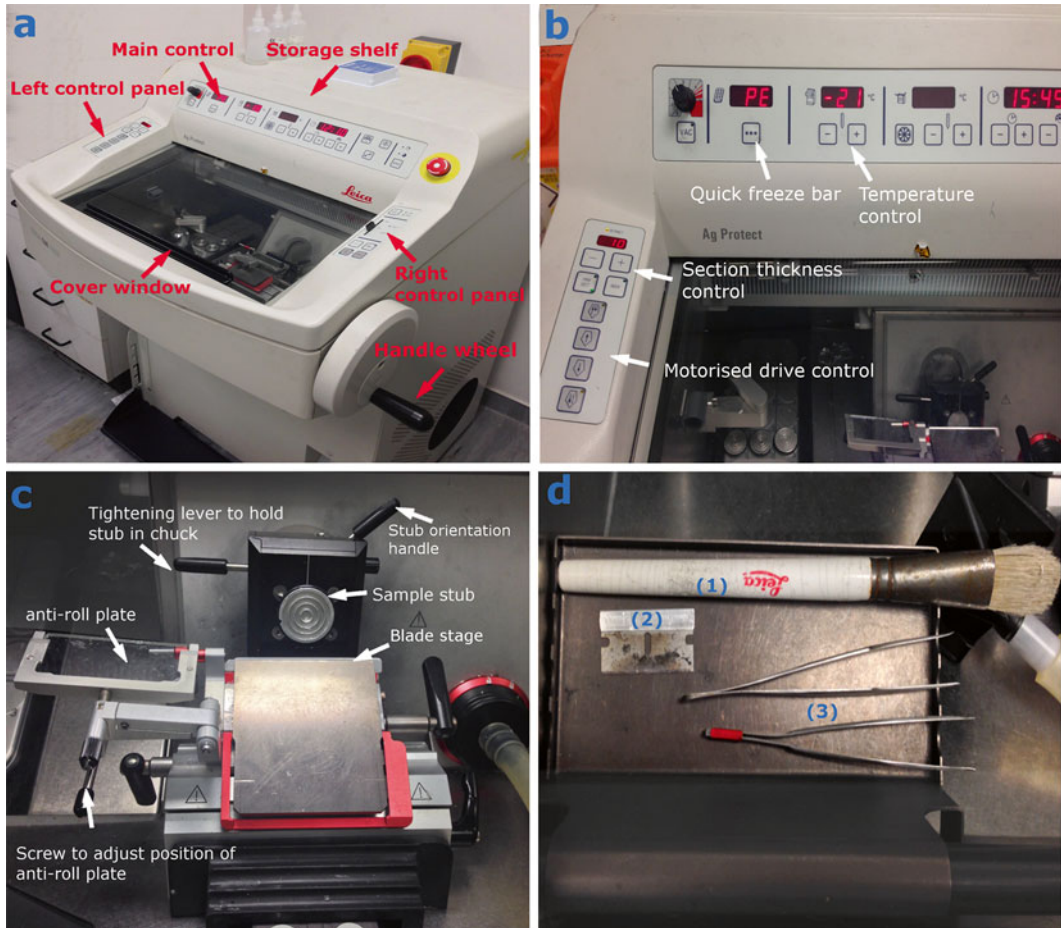
Fig. 3 Cryostat cross-sectioning of skeletal muscle. (a) A Leica CM1950 cryostat with parts labeled. (b) Detail of cryostat control panels. (c) Detail of stub sample holder and blade stage, with adjustment controls highlighted. (d) Equipment required for sectioning. (1) 13 mm brush, (2) mounted razor blade, and (3) fine forceps
