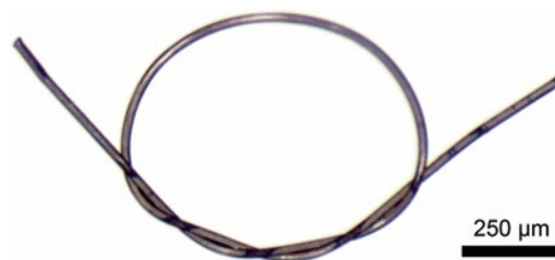
Fig. 3 Loop of USP 10-0 monofilament nylon suture used to attach the fiber to the experimental apparatus. Note that the knot type is double-overhand, not single-overhand. Reproduced from Roche et al. 2015 [4] with permission from JoVE
