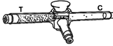
Fig. 1 T-maze apparatus [25] is modified from [56] in that a two-way plug is substituted for the original three-way plug. Test solution is in the T arm; control solution in the C arm; cells are loaded through the remaining arm. Cells are allowed to move through the T-maze for 30 min after the plug is turned to allow them access to the C and T arms. After 30 min, the plug is turned, arms emptied and cells counted
