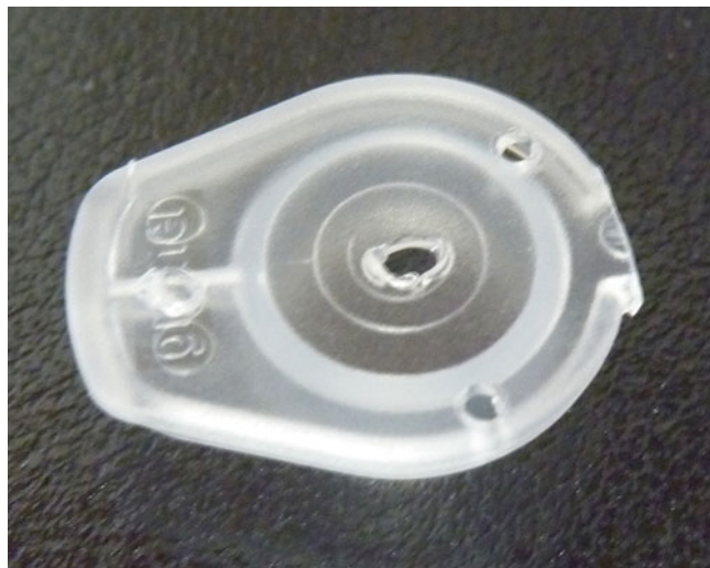
Fig. 3 Polypropylene cap from a microfuge tube containing three holes for a suture, and one central hole for transplantation
