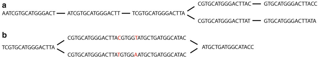
Fig. 2 (a) An example De Bruijn graph with k-mer size 16 and 5 nodes. (b) A bubble caused by two SNPs or sequencing errors. Shorter k-mers will decrease bubble size, but could increase fragmentation if coverage is not high enough
