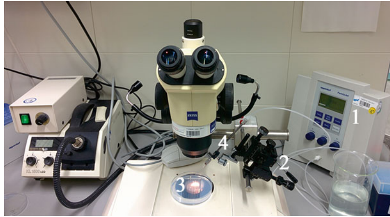
Fig. 4 The basic zebrafish microinjection system. (1) Microinjector with air pressure. (2) Micromanipulator. (3) Agarose plate with one or two-cell stage embryos. (4) Needle holder
