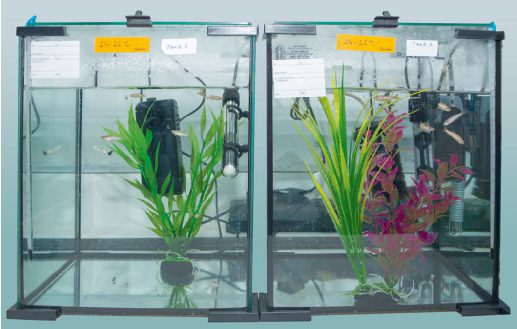
Fig. 2 An example of the glass tanks used for temperature shift experiments. Separate glass tanks are filled with system water and contain filters and heaters to control the water quality and adjust the temperature. Additional thermometers are placed inside each tank to monitor the temperature. Each tank is also labeled with information regarding the fish and temperature settings
