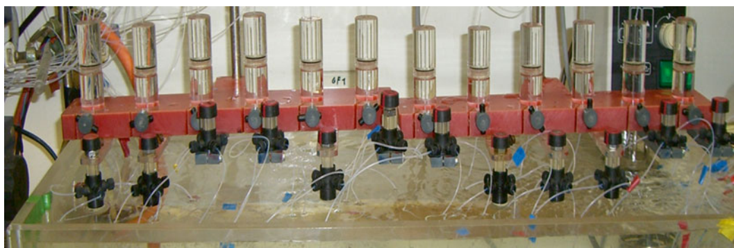
Fig. 3 Twelve-channel superfusion apparatus. Note that the valves in front allow for rapid and simple exchange of solutions, i.e., from baseline buffers to drug containing buffers. The tubing is typically immersed in a water bath, which should be kept at a temperature higher than the desired value in the chamber
