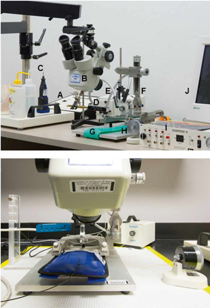
Fig. 4 Experimental set-up. Upper panel showing, A potentiostat, B dissecting microscope on boom stand, C dremel tool, D headstage, E light source, F stereotaxic frame, G water-circulated heating pad, H microdrive, I picospritzer, J monitor (and computer, out of picture). Lower panel , showing a closer view of headstage, stereotaxic frame, water-circulated heating pad, microdrive, and dissecting microscope, which is used both during surgical preparation of the animal, and for measuring the fall of meniscus in the micropipette
