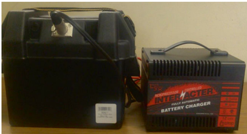
Fig. 10.1 External ventilator battery with charger
