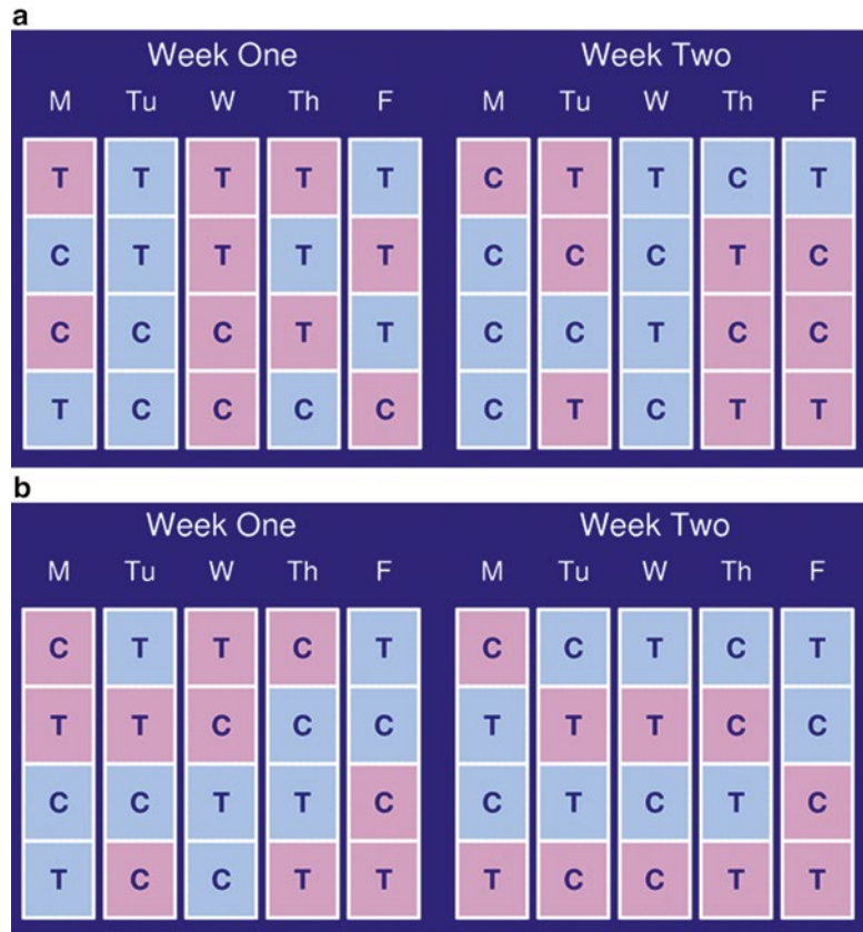
Fig. 1 (a) Treatment allocation from a completely randomized design; (b) treatment allocation from a randomized complete block design. T =treated, C =control, pink =female, blue =male
