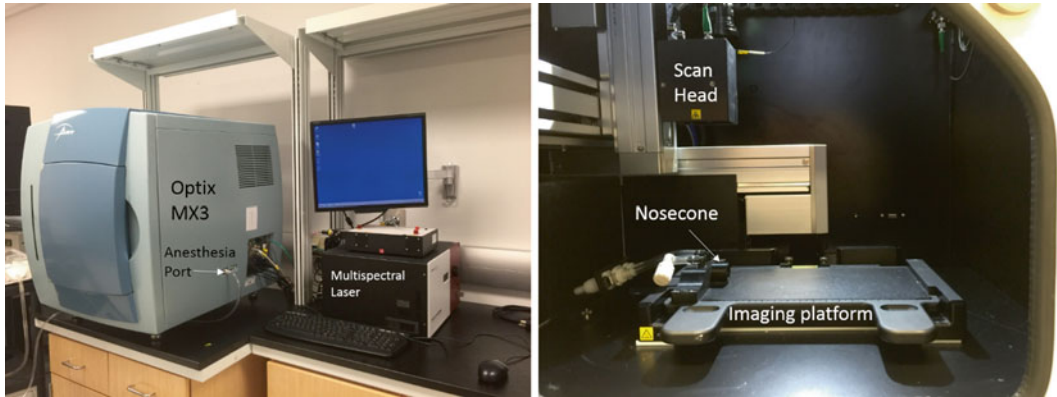
Fig. 3 Optix MX3 time domain diffuse optical imaging system equipped with supercontinuum white light laser, gas anesthesia, and heated imaging platform for imaging mouse models of cancer
