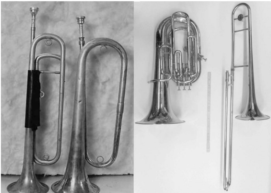
Fig. 8.13 Two examples of brass instrument families, each having one cylindrical bore instrument and another with a conical bore. Left : trumpet ( cylindrical ) and bugle ( cone ). Right : trombone ( cylindrical ) and low saxhorn ( cone )
