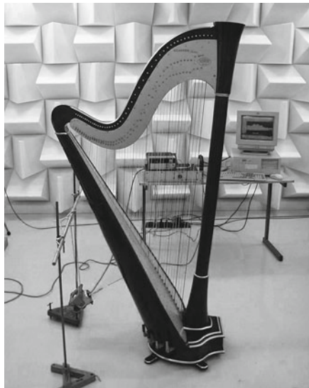
Fig. 3.18 (Left) Excitation of sympathetic strings. Several strings which have one end fixed to a moving bridge are likely to vibrate in sympathy. Such a phenomenon requires two conditions: the transfer admittance between i and j should not be zero, and the strings must have at least one eigenfrequency in common. (Right) The harp is an example of instrument where sympathetic vibrations are observed, because of the coupling of the strings through the mounting bar located on the axis of the soundboard [24]
