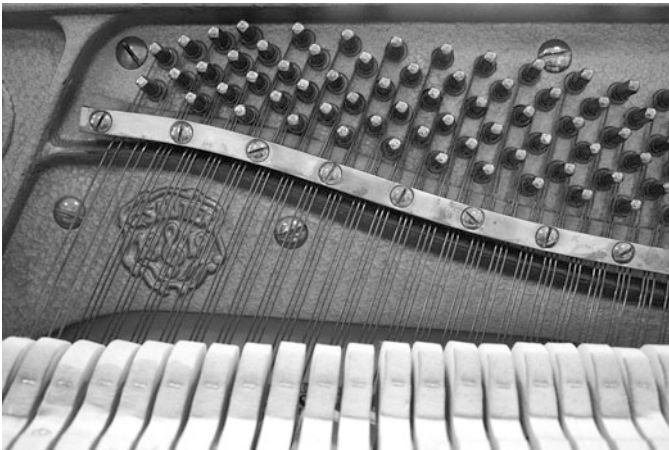
Fig. 6.6 Inside view of a piano showing string doublets ( far left ) and string triplets struck by the same hammer. © Pleyel
