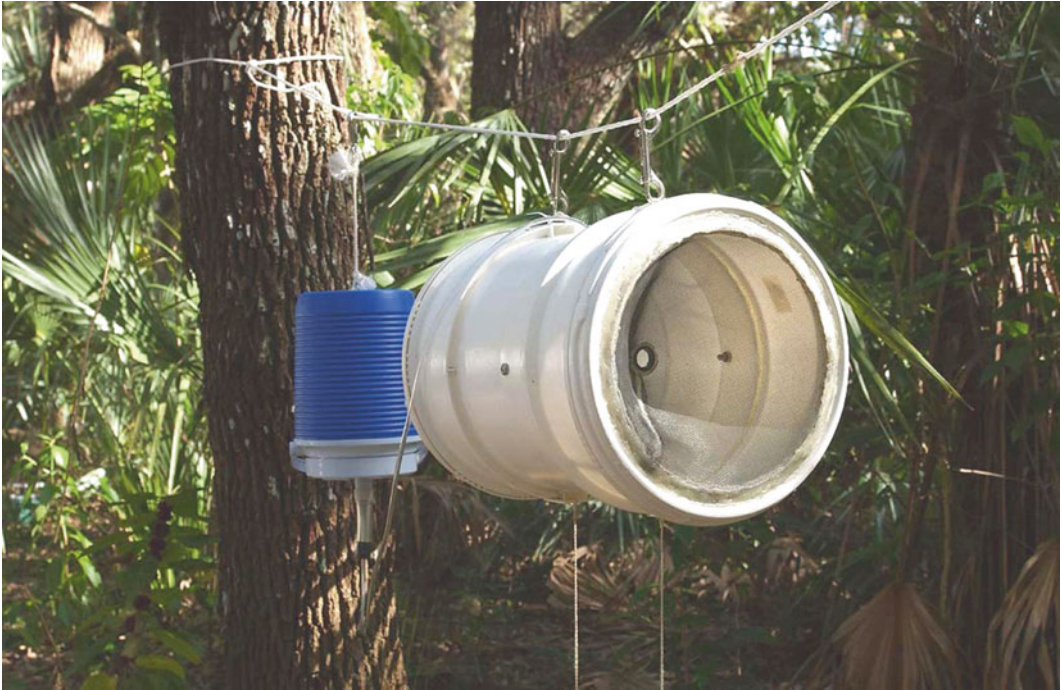
Fig. 2 Photograph of an unmodified lard can trap (foreground) that is properly deployed. This collection is baited with dry ice contained in the blue cooler (background). Carbon dioxide is released from a simple tube connection between the cooler and the interior of the trap. Photo credit: Jim Newman, University of Florida—Florida Medical Entomology Laboratory
