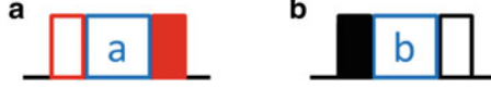
Fig. 3 The pulse sequence of single spin operations. (a) Corresponds to the Eq. (58). (b) Corresponds to Eq. (62). Dotted blocks of a and b are the \theta = 2\alpha rotation around the x - and y -axes, respectively
