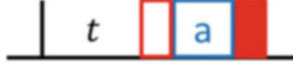
Fig. 6 Generation of \exp(-i\hat{H}^{zz}\Delta t/\hbar) by the spin rotation around z -axis in the case of Eqs. (86) and (61). The dotted block a is the spin rotation around x -axis which spin number and angles ( \theta^k ) are shown in Table 1
