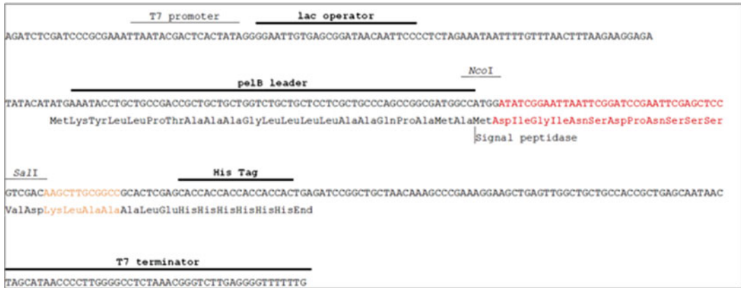
Fig. 3 pET-22b(+) DNA and amino acid sequence in the area where the ortholog DNA is inserted. Areas of interest are marked. The red DNA and amino acid sequence were replaced with the target DNA. The orange amino acids were removed and replaced with the DNA sequence for TEV protease cleavage sequence ENLYFQS. Image was adapted from that available from Novagen website
