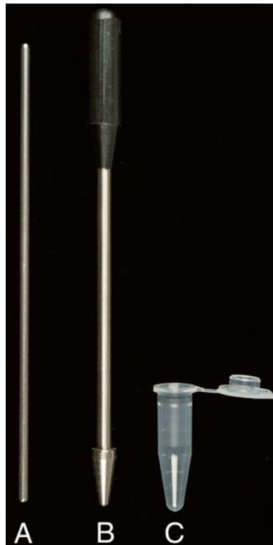
Fig. 2 Equipment for maceration as described in see Note 1 . (a) Stainless steel rod with flat end. (b) Stainless steel grinder made to the internal profile of an Eppendorf tube (c)
