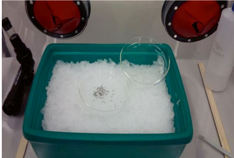
Fig. 2 Glove box set up showing tray of ice, anesthetized mosquitoes in a petri plate, ethanol bottle, and D-cell aspirator. (Photo J.P. Ledermann)
