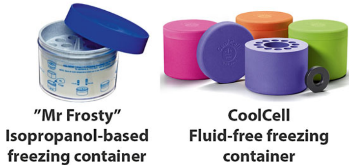
Fig. 2 Freezing containers. The traditional “Mr. Frosty” isopropanol-based freezing container, where the isopropanol must be changed every few uses to ensure the controlled rate -1\text{ }^{\circ}\text{C}/\text{min} . CoolCell fluid-free freezing container is easy to use and provides a highly reproducible -1\text{ }^{\circ}\text{C}/\text{min} freezing rate when placed in a -80\text{ }^{\circ}\text{C} temperature
