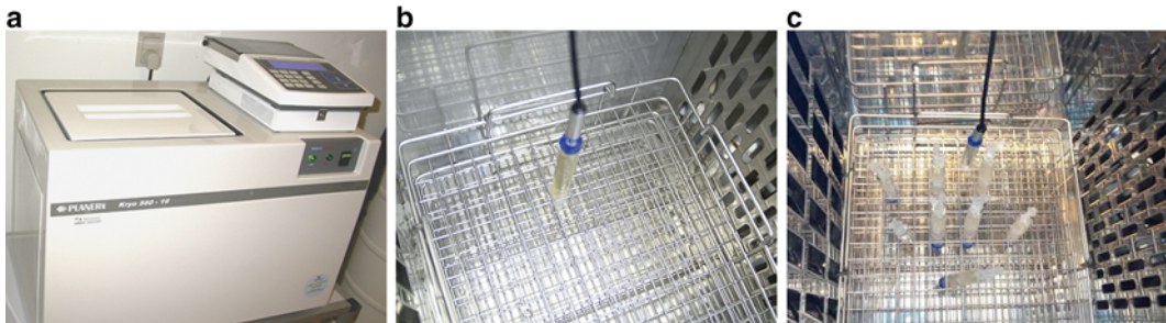
Fig. 5 Cell freezing. (a) Programmable controlled-rate freezer. (b) Temperature probe is attached to control freezing vial. (c) All the CellSeal vials with cell suspension are placed into the freezer
