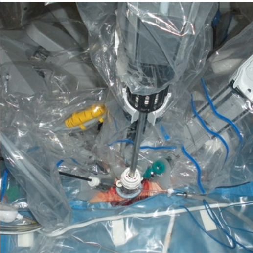
Fig. 5.2 Setup for robotic LESS prostatectomy using the da Vinci® Si platform and the SILS® multichannel port
