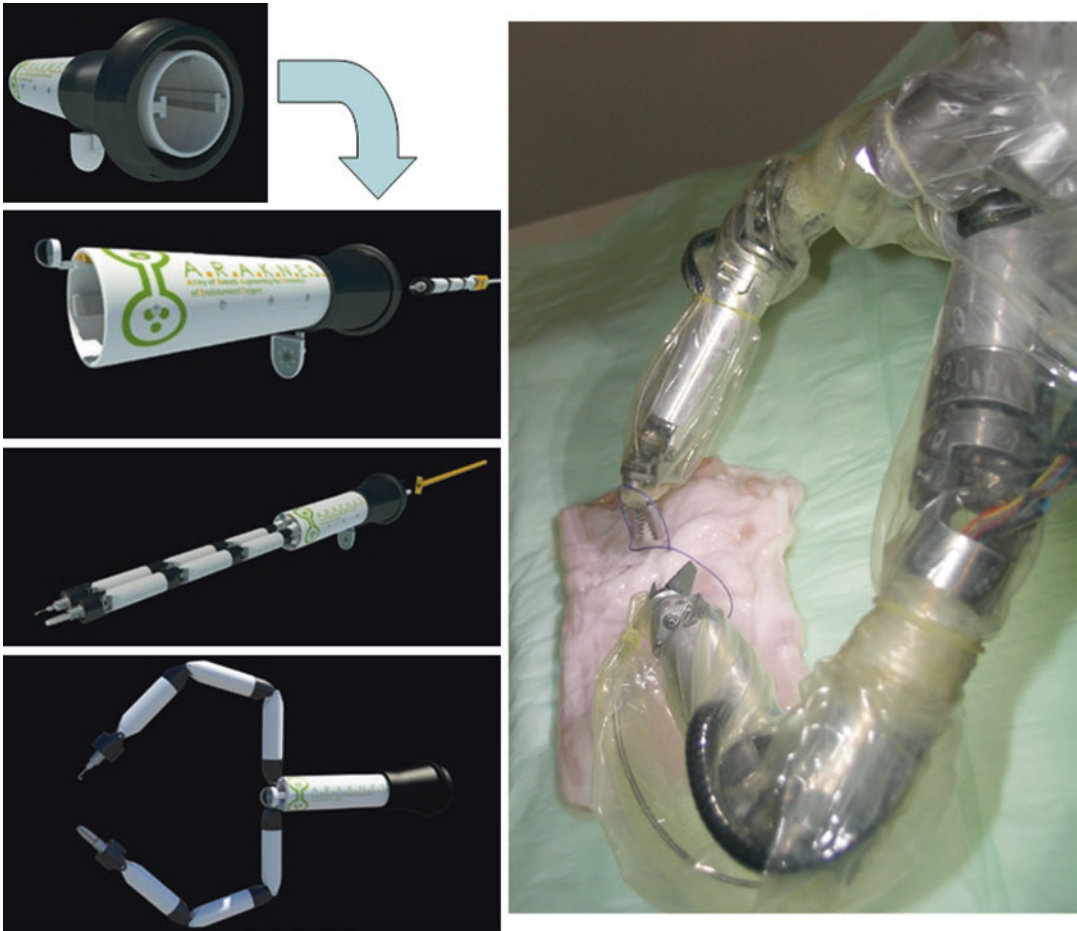
Fig. 5.8 SPRINT robot. (a) Illustration of the insertion sequence into the patient abdomen: umbilical access port with the introducer, insertion of the first arm through the
