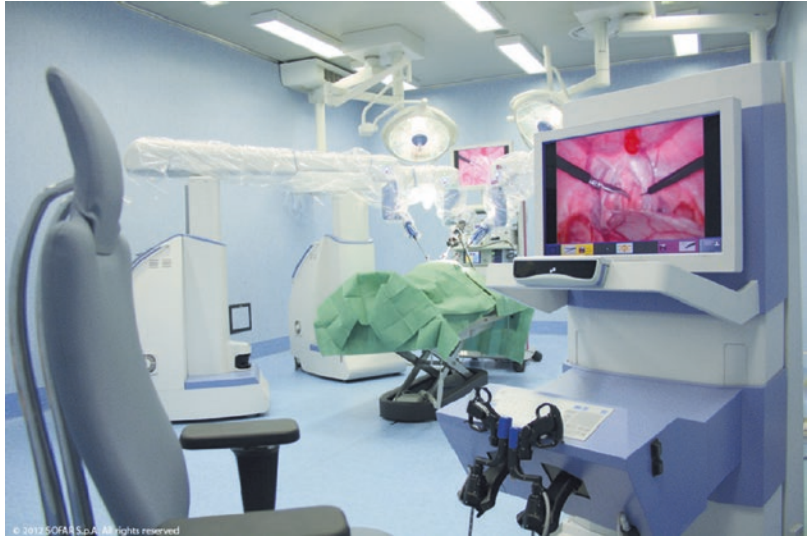
Fig. 5.9 ALF-X (Advanced Laparoscopy through Force-RefleCT(X)ion) (Courtesy of SOFAR spa)
