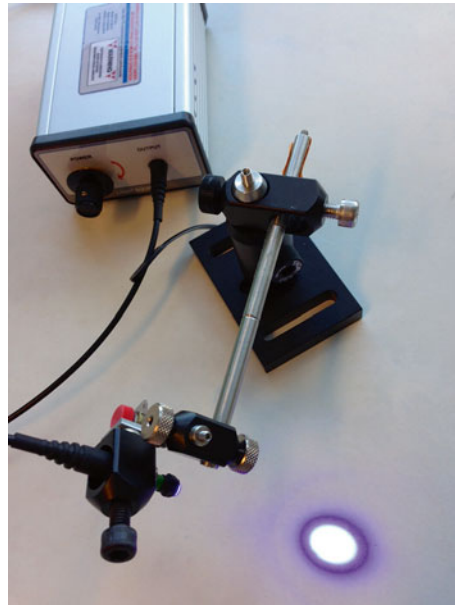
Fig. 5 Alternative mounting of fiber-coupled LED using posts and clamps with fitted miniature collimator. Maximum illumination intensity for demonstration
