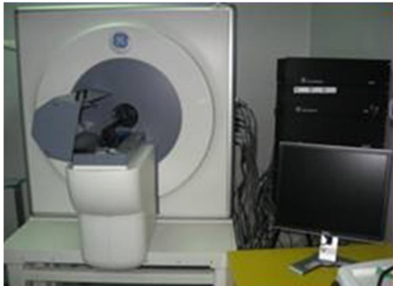
Fig. 8.4 High-resolution computed tomography (CT) instrumentation for small animals (<50 \mu m). This system uses an X-ray detector with a kV range of 35–80 and an mA range of 0–500. The system has three isotropic resolution settings (27, 45, and 90 \mu m) with a field of view (FOV) up to 80 mm in diameter. The Locus system uses a CCD with 10- \mu m square detector element and 100 mm \times 50 mm active area. The scan time is 5–60 min depending on the protocol used, with sensitivity in the order of millimolars
