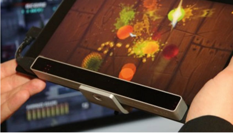
Fig. 3.5 Low-cost eye-tracking device here attached to a tablet (here the Eye-tribe system)
