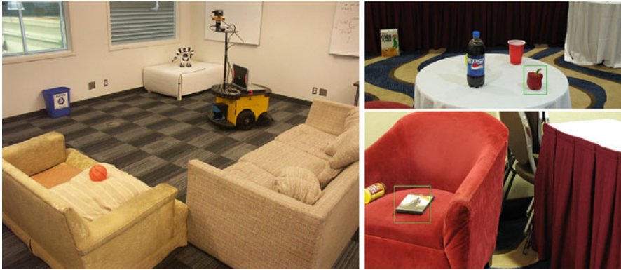
Fig. 21.12 Left: the robot Curious George within the room it is exploring. Right: two objects detected and successfully recognized by Curious George. (Reprinted with permission from [42])
