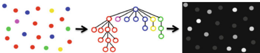
Fig. 9.14 ESAL algorithm on a color synthetic image. From left to right: the synthetic image, the tree where each node is colored according to the corresponding candidates, the computed saliency map based on self-similarities (Adapted from [17])
