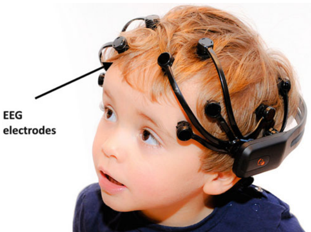
Fig. 3.11 A low-cost commercial EEG (here the Emotiv EEG system)
