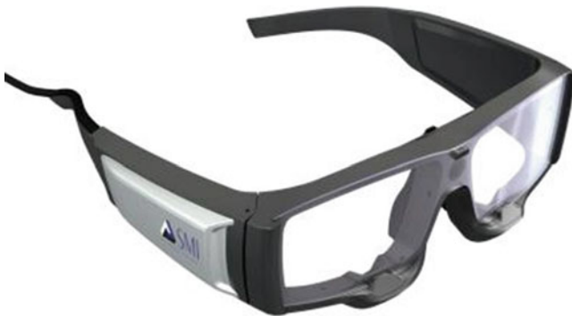
Fig. 3.4 Eye tracking embedded in wireless (here a SMI system)
