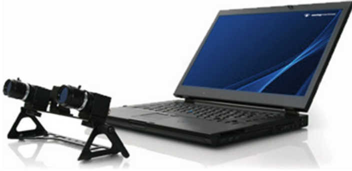
Fig. 3.3 Binocular eye-tracking system independent from the screen (here a Facelab system)
