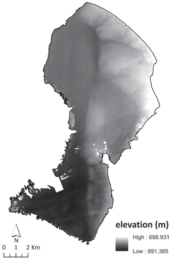
Fig. 2 Standing water volume was calculated using the LiDAR-derived DEM underlying the extent of water identified in the imagery. Elevation ranges from ~691 to ~699 m for the lake bed
