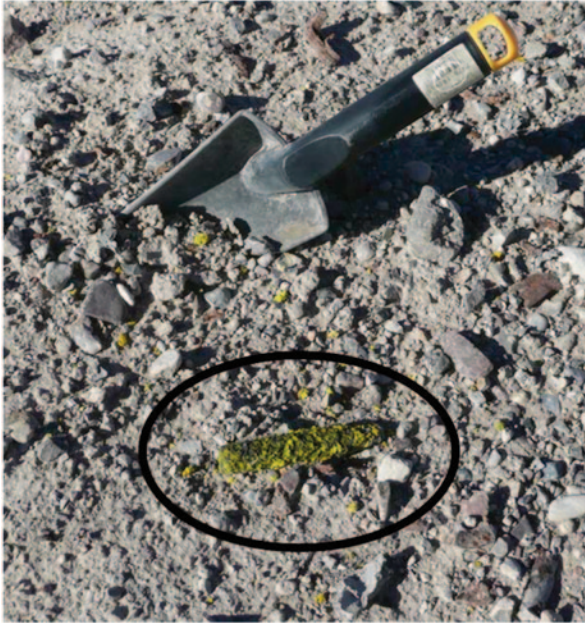
Fig. 1 The growth of DU oxides on the surface of the DU projectile ( circled ) results in a stippled appearance of the projectile. The DU oxides that have been eroded from the projectile surface are scattered on the surrounding ground
