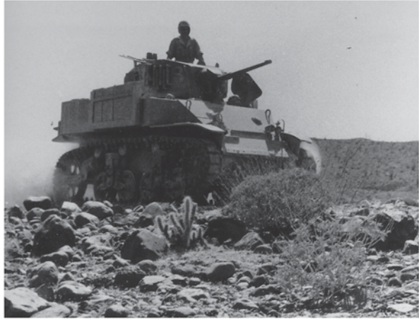
Fig. 3 Stuart Light Tank undergoing testing at Camp Seeley. Note the side mounted racks with concrete blocks to increase test weight of vehicle. (Photo from Heritage Center of YPG)
