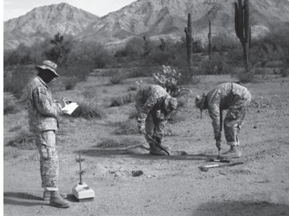
Fig. 3 Cadets collect data with a Nuclear Density Gauge in Yuma, AZ
