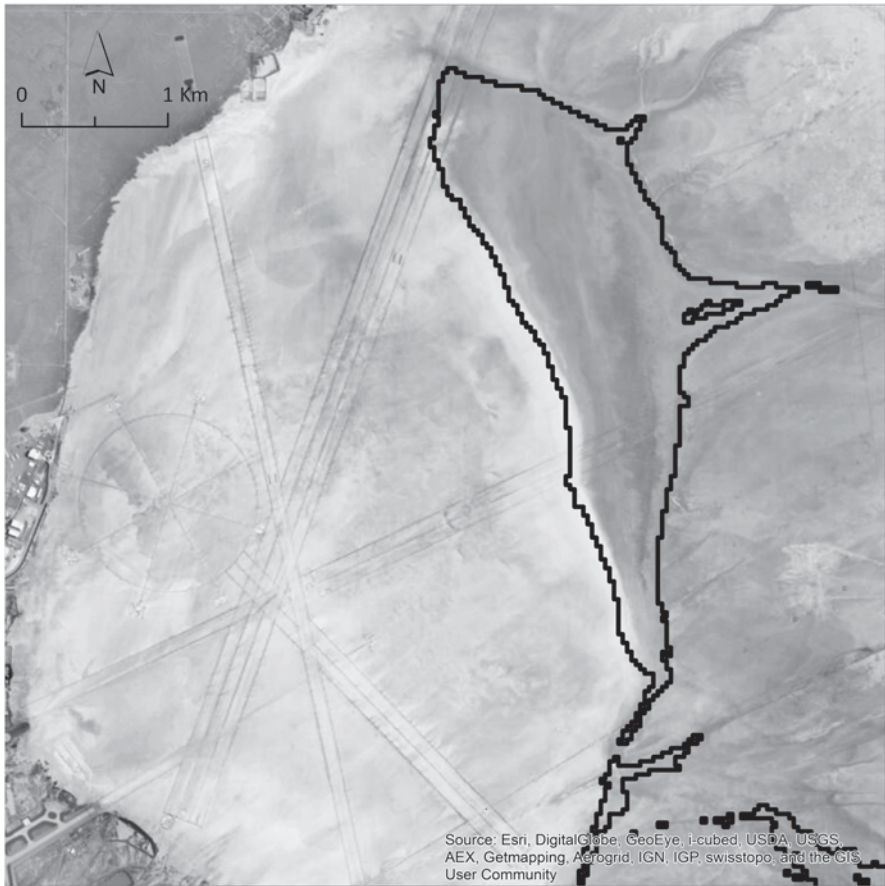
Fig. 4 Runways and surface water extent mapped from the 7 March 2003 imagery ingested in Google Earth Pro (© 2012 Google, © 2012 TerraMetrics) over the northwestern extent of Rogers Lake. This illustrates the utility of assessing where water, outlined in black, covered parts of runways following the February 2003 storm event and could be used in predictive modeling
