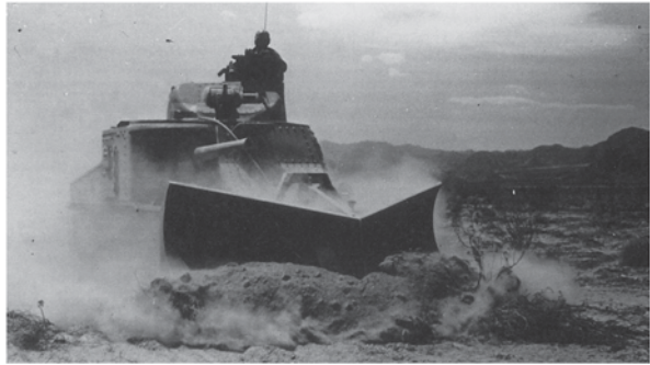
Fig. 2 M3 Lee tank fitted with experimental blade at the DTC. (Photo from Heritage Center of YPG)
