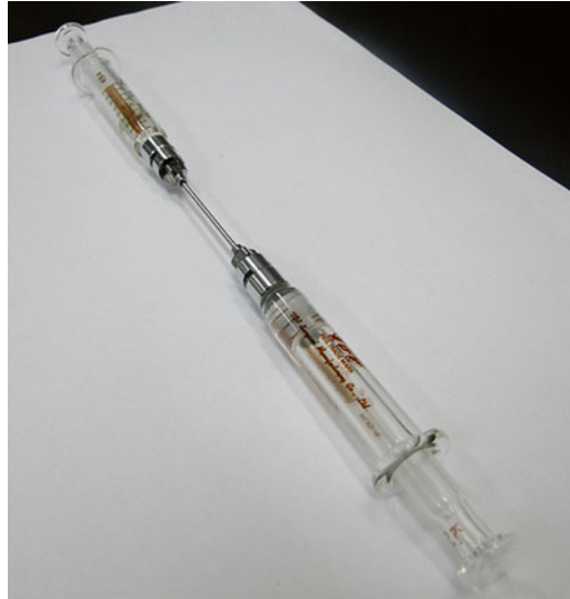
Fig. 1 Two syringes, one containing recombinant protein and the other containing adjuvant, connected by a micro-emulsifying needle
