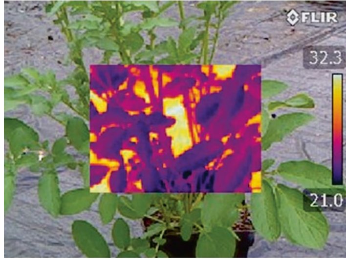
Fig. 2 Example of data fusion from FLIR camera E50 with Picture in Picture available on the camera's LCD for identification and distinguishing foreground and background component elimination while screening/phenotyping
