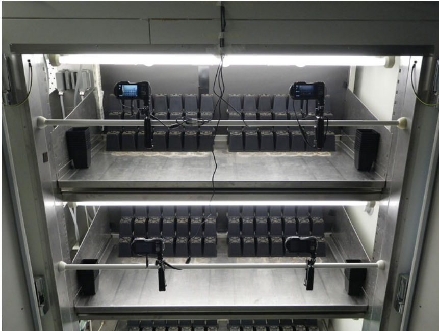
Fig. 1 Overview of the imaging system. Pentax Optio WG-1 cameras are fixed to shower curtain rods with clamp tripods. Twenty-seven 7 \times 7 cm pots can be placed on the pot stands in front of each camera allowing imaging of 108 tomato seedlings using four cameras
